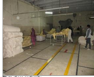
Photo of non-conformity NC spot cleaning area in finishing department was not isolated with other production area.JPG
